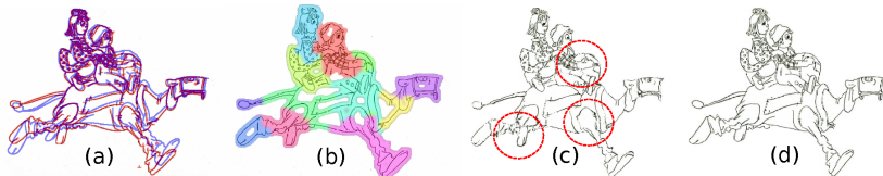
Fig. 1. Cartoon sequence. (a) 1st (blue) and 4th (red) frame. (b) Groups found by our algorithm of Sec. 3.2. (c) TPS interpolation with artefacts enclosed in a circle (e) Our piecewise affine transformation using the found groups.
