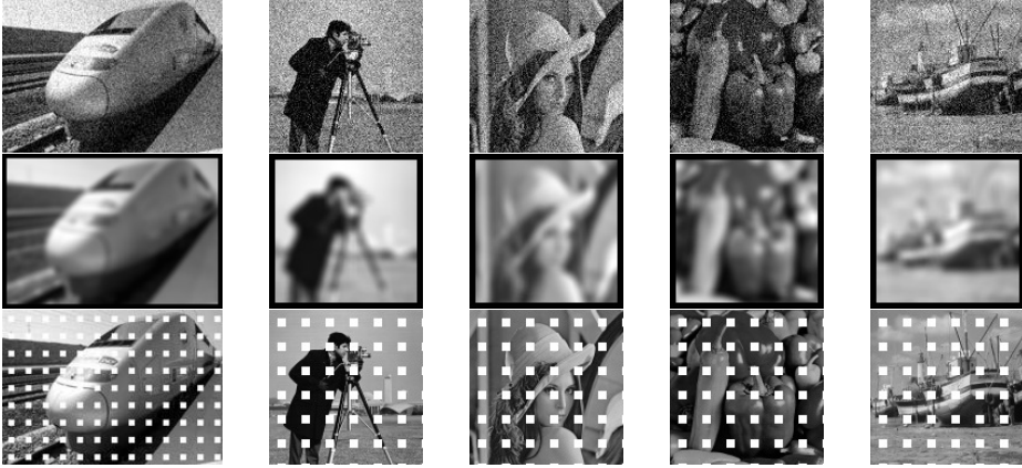
Fig. 1. Test images used for evaluation. Top row – denoising: with additive Gaussian noise (zero mean, standard deviation 0.1). Middle row – deblurring: blurred images with Gaussian noise (zero mean, standard deviation 0.01). Bottom row – inpainting: white regions mark the regions to be inpainted.
