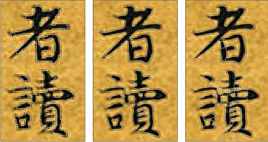
Figure 7.46: Segmentation results on two characters from the fragment shown in figure 7.45 (computed on the red channel of the original color image, and using two-fold oversampling in case of the subpixel-accurate detectors). Left: Pixel-accurate thresholding (threshold t = 13 ). Center: Subpixel-accurate thresholding (threshold t = 13 ). Right: Subpixel watersheds of the gradient magnitude ( \sigma_{\text{filter}} = 0.8 , gradient threshold g_0^2 = 1.4 ). Algorithm parameters apply to the noise normalized red channel.
