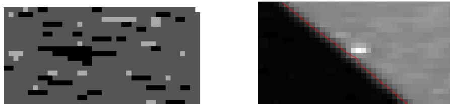
Figure 7.31: Examples for non-Gaussian noise in the “benchmark1” set (image “d2”). Left: Contrast enhancement in the dark image region reveals horizontally correlated quantization noise. Right: Outliers near the true contour cause distortions in the detected edge. Horizontal noise correlation is also visible in the bright image area.
