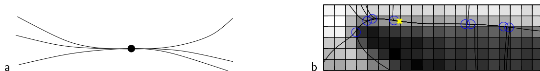
Figure 5.5: Tangential watershed convergence at a local maximum. Top: illustration; bottom: actual watersheds on an image – the single maximum of the boundary indicator in the ROI is marked yellow, and the blue circles mark locations where the half-edges converge (precisely, the r -circles where the \sigma -order is eventually found).
