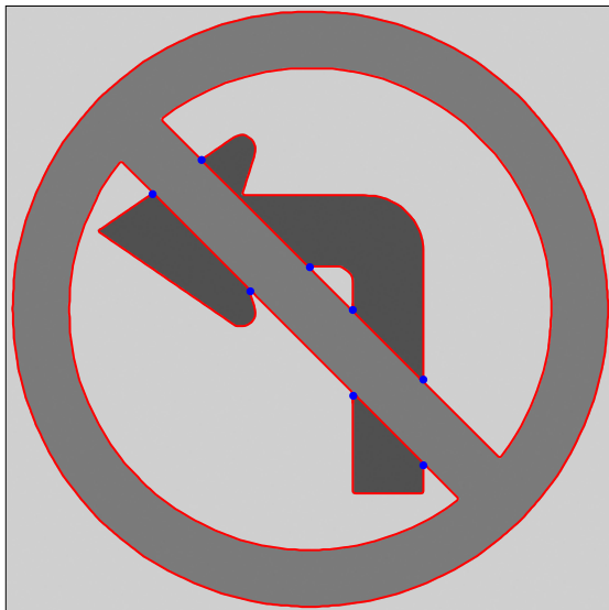
Figure 4.7: A polygonal GeoMap that encodes the partition of the image shown in the background (red: arcs, blue: vertices).
