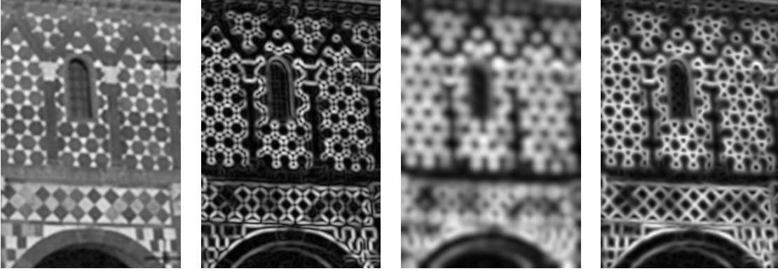
Figure 9.2: Left: The facade of the entrance hall of Lorsch monastery is decorated with delicate tilings. Center left: The gradient magnitude correctly represents the edges of the tiles, but is zero at their corners (because these points happen to be saddle points, i.e. the gradient vanishes). Center right: Due to excessive blurring, the tiling structure is lost in the square root of the structure tensor trace. Right: The square root of the trace of the anisotropic structure tensor (i.e. integration is done with the hourglass filter) represents both edges and corners correctly. Parameters were \sigma_{\text{filter}} = 0.8 , \sigma_i = 1.6 , \sigma_\phi = 0.4 . All computations were performed in a two-fold oversampled image to avoid aliasing artifacts (cf. section 7.1), and the given filter sizes have been scaled accordingly.
