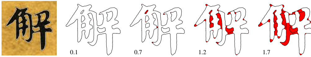
Figure 5.16: Left: Boundary detected for a Chinese character using the subpixel thresholding algorithm 5.2. Right: As \alpha is increased, the (\alpha, \beta) -boundary reconstruction becomes thicker, indicating increasing uncertainty about the true boundary location.
