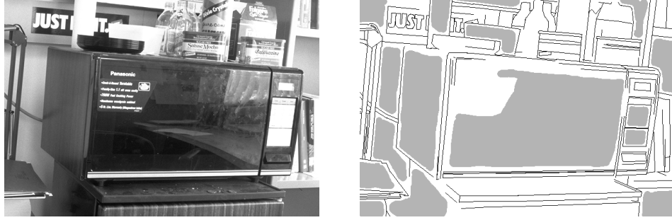
Figure 2.15: Image 50 (left) from the University of South Florida edge detector evaluation data set and the corresponding ground truth image (right) with “no edge” (gray), “edge” (black), and “don’t care” (white) labels.
