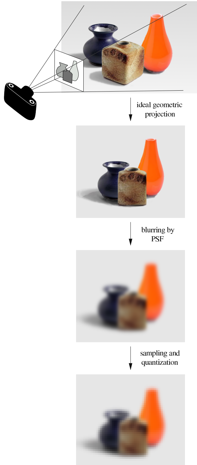
Figure 3.1: The image acquisition model employed in this work (compare figure 2.1).
