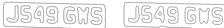
Figure 1.3: Segmentation of the license plate with the subpixel watershed algorithm (left) and the subpixel zero-crossing algorithm (right) after twofold oversampling. See chapter 5 for a description of these methods.
