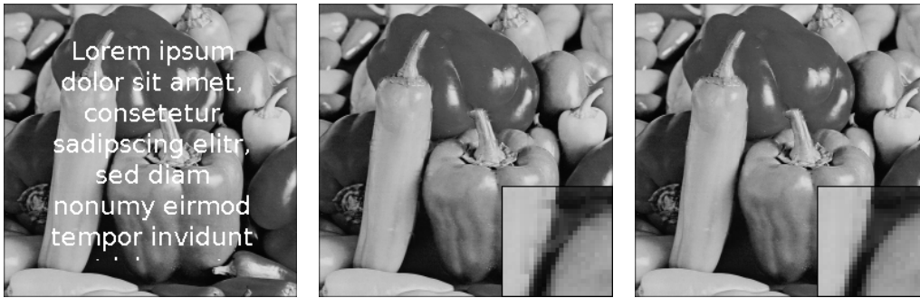
Figure 5. Prototypical use of the proposed software framework for the problem of image inpainting (Sect. 3.2). We used a simplified framelet approach [5] without sub-sampling. The underlying mathematical problem of recovering the white regions ( left ) can be modelled efficiently using COAL (Fig. 3). Variants such as replacing the least squares objective ( middle ) by a robust Huber kernel ( right ) can be evaluated by changing a single line of code.
