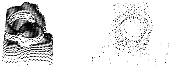
Fig. 2 Examples of 3D point cloud models obtained by a sample scan (left) and by discretizing a CAD model (right).
