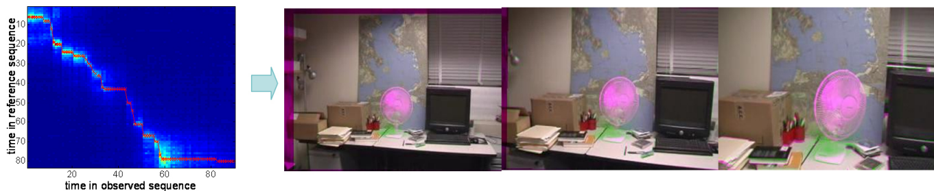
Fig. 5. From left to right: the joint video alignment energy computed by Eq. (8) inside the range defined by time (frames) x_i in reference sequence/ time (frame) i in observed sequence. The red line is the most likely frame correspondence x_{1:n_o} = [x_1 \dots x_{n_o}] found using Algorithm 1. Example results of our approach on 'indoor-1' pair provided by Sand and Teller [3] in order to illustrate some representative results.
