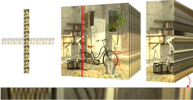
Figure 2: Extraction of an Epipolar-Plane Image (EPI). The vertical views captured by a cross light field (left) are stacked (middle). A slice through a column (right) forms an EPI (bottom). Note, how the slopes of lines in the EPI encode the three-dimensional structure of the scene.
