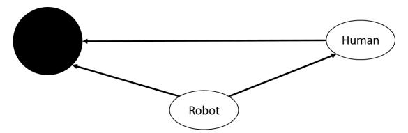
Figure 4.2: Experimental setup with a human moving towards a hole and a robot trying to protect the human
